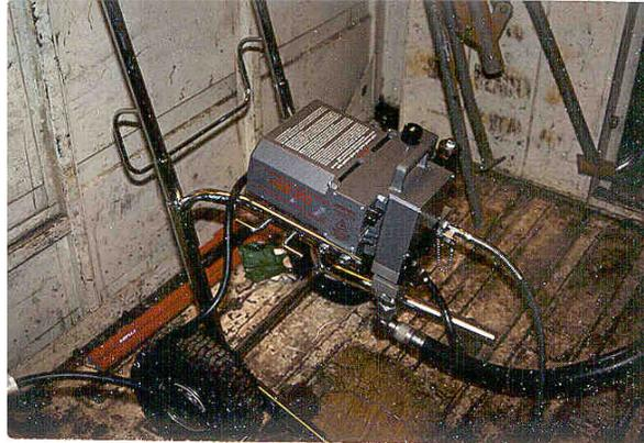
*Typical single stage polyurethane chemical grout piston pump*
